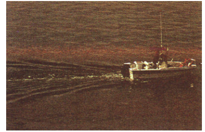
Fig. 16-22 The passing of the leading edge of a boat's wake is the water wave equivalent of a sonic boom and is created when a boat moves through water at a speed greater than that of the waves it produces.
