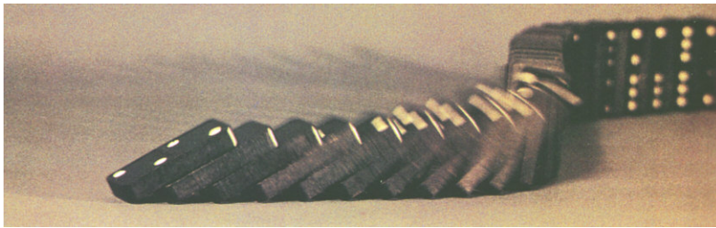
Fig. 16-1 When the domino at the left end of this line is pushed over to the right, a wave pulse passes through the line.
