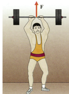
Fig. 7-25 A weight lifter provides a nonconservative force \mathbf{F} , doing positive work and increasing the weight's mechanical energy.
